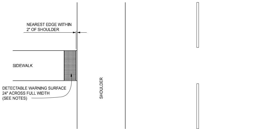
DETECTABLE WARNING AT FLUSH SHOULDER OR ROADWAY
